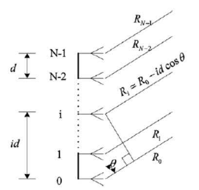
The transmitter signals received by adjacent antenna elements have a phase difference of  $2\pi \frac{d \cos \theta}{\lambda}$ , which allows us to obtain the bearing of the transmitter from the measurement of the phase difference.
