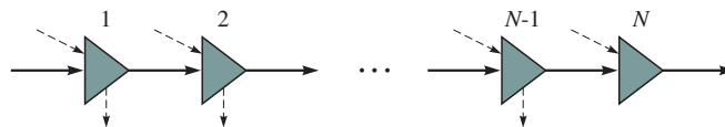
FIGURE 7.41 The end-to-end QoS of a packet along a path traversing N hops
