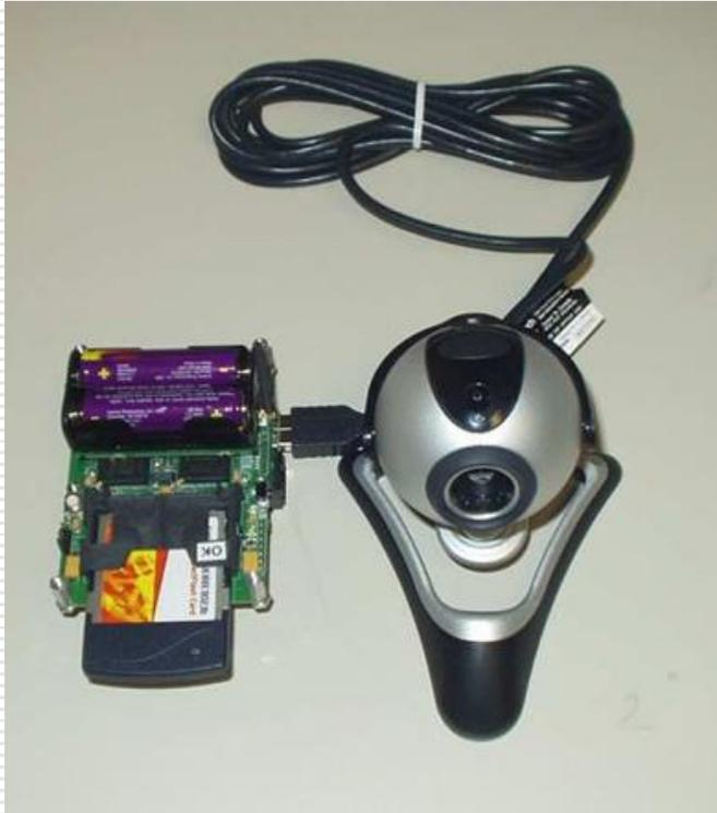
Stargate board interfaced with a medium resolution camera.
