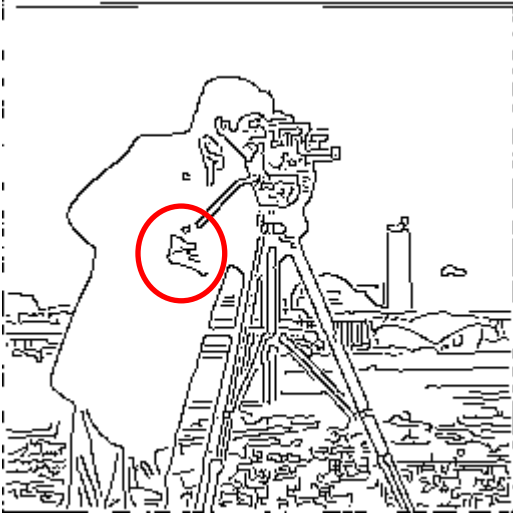
Fig. 11. Result of applying the gradient-based extension of Demigny's filter with W=2 and \sigma=2 to Fig. 2.
