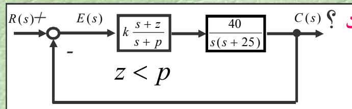
3- Locate the compensator pole so that the angle criterion is satisfied.
