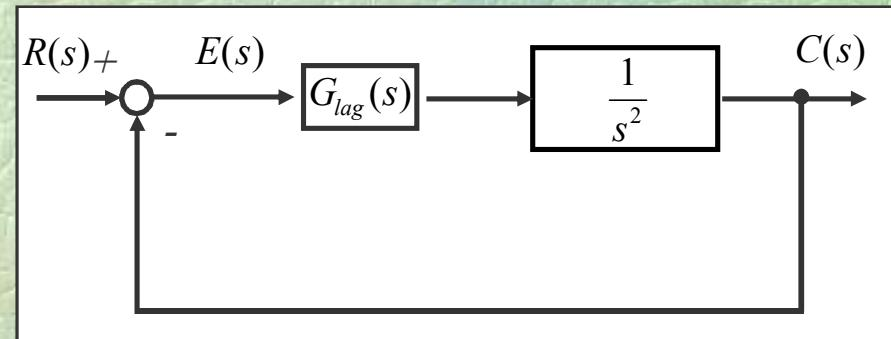
6 In the following system design a lead controller such that that the settling time be less than 3 sec.
