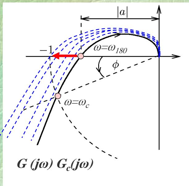
We define **gain margin** as the **gain** that the frequency response would have to increase to move to the -1 point.
