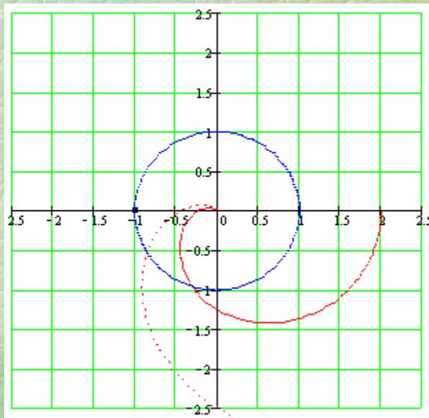
The two different Nyquist plot above would lead to two different phase margins. The system with the frequency response with the dashed line is less stable.
