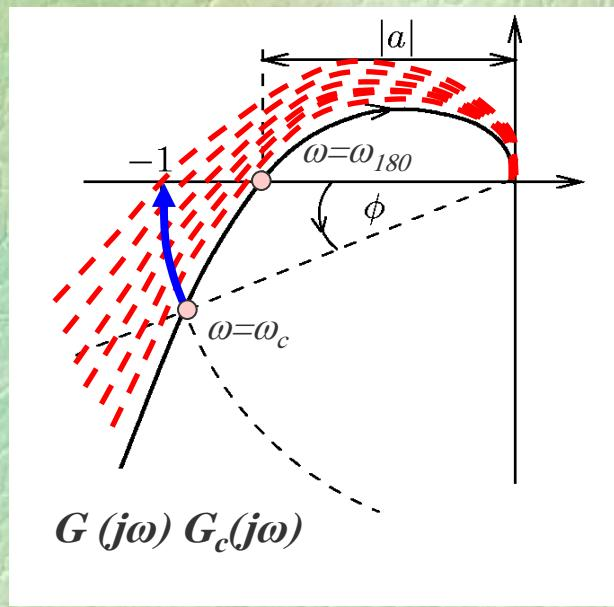
We define **phase margin** as the **phase angle** that the frequency response would have to change to move to the **-1** point.
