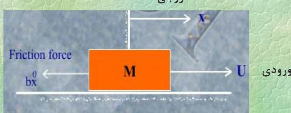
$$u - b x = M \ddot{x} \rightarrow \ddot{x} + \frac{b}{M} x = \frac{1}{M} u \quad , \text{with } a = x$$
