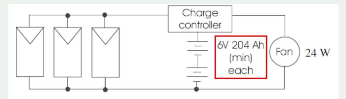
24 W during a day  $\rightarrow$  24×24 = 576 Wh Using 12 V batteries  $\rightarrow$  576/12 = 48 Ah Batteries efficiency  $\rightarrow$  48/0.9 = 53.3 Ah Wiring efficiency  $\rightarrow$  53.3/0.98 = 54.4 Ah Let three day with no sun  $\rightarrow$  54.4 × 3 = 163 Ah Let 20% deep of discharge  $\rightarrow$  163/0.80 = 204 Ah<sub>10</sub>
