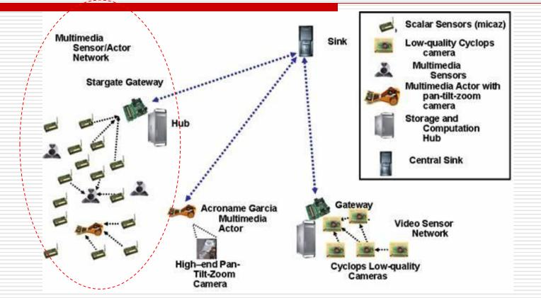
Transmitting multimedia streaming data in wireless sensor networks
