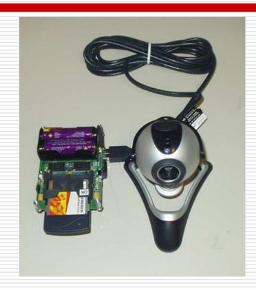
Stargate board interfaced with a medium resolution camera.
