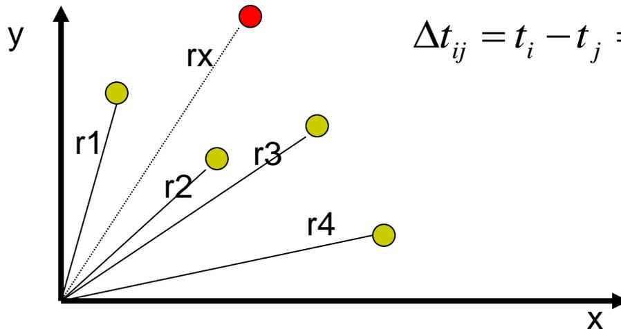
$$\Delta t_{ij} = t_i - t_j = \frac{1}{c} (\|r_i - r_x\| - \|r_j - r_x\|)$$
